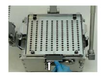
**6.** Press release bar to drop the tablets into the capsules.
