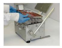
6. Place Caplet Tray on Caplet Orienter Base and slide back until it drops into place.
