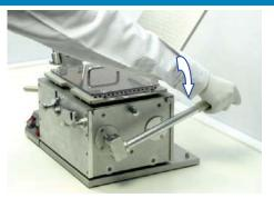
3. To separate size AAel capsules, see Inset 1 on next page. For other capsule sizes, <u>slowly</u> push down Lifting Handle just until capsules separate. As soon as you begin to feel resistance, <u>slowly</u> release the Lifting Handle. This resistance occurs as the Bottom Plate begins to lift the capsule bodies. Continuing past this point will cause the capsule bodies to be lifted out of the Filler. See Capsule Separation Tip below.
