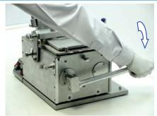
After inserting trial product or filling powder, follow the instructions in the ProFiller 3700/3800 Manual Operating Instructions for "Locking Capsules" (page 20 in Manual v 1.2.1).
