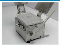
**3.** Place the Capsule Orienter Base on the OE Guide Tray. Align the front edge of the Orienter Base with horizontal line I on OE Guide Tray. Align the right edge of the Orienter Base with the right edge of the OE Guide Tray.
