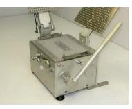
**2.** Place the OE Guide Tray onto the Filler. Steps for caplet orientation are similar to capsule orientation.
