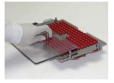
**5**. Set Caps Tray with Push Plate on table. <u>Slide</u> Push Plate off Caps Tray to avoid lifting caps due to static.
