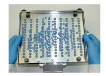
**3.** Pour tablets onto ATF and tilt in all directions moving capsules into slots.
