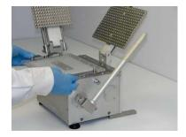
9. Remove the Caplet Orienter Base, Caplet Trav and OE Guide Tray. Continue with Operating Instructions in your ProFiller 3700/3800 Manual. Begin with "Filling Capsules" if adding an excipient (page 18 in Manual v 1.2.1), or continue with "Locking Capsules" to lock the outer capsules (page 20 in v 1.2.1).
