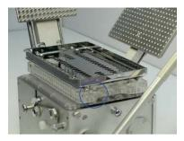
7. Push sliding portion of Caplet Tray to the left 8. For all sizes, move the Caplet Orienter Base with Caplet Tray to position II on OE Guide Tray. Repeat steps 4-7.
