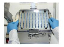
**5.** Place ATF locating studs into <u>front</u> holes of OE Guide Tray.
