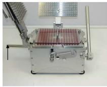
1. Make sure Cam Handle is at  $0^\circ$  on cam indicator. Place loaded Caps Tray with Push Plate onto Filler.
